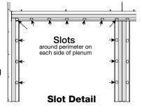
Tighten the bolt-washer assemblies to the top and both sides of the joining sections. Start on the lower sides and work towards the top. As the bolts are tightened, the plenum sections will draw together. Use anti-seize gel to prevent galling / welding of all stainless steel fasteners. If necessary, pull the units together with a mechanical come-along device at the structural base of the unit or at lifting lugs.
